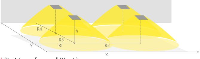
R1 distance from wall (X axis) R2 installation distance between lights (X axis)
