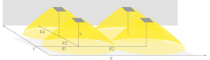
R1 distance from wall (X axis) R2 installation distance between lights (X axis) R3 installation distance between lights (Y axis) R4 distance from wall (Y axis) Y9292WM
