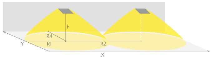
R1 distance from wall (X axis) R2 installation distance between lights (X axis) R4 distance from wall (Y axis) Y9292WM
