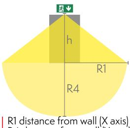
R1 distance from wall (X axis) R4 distance from wall (Y axis) Y9051WK120
