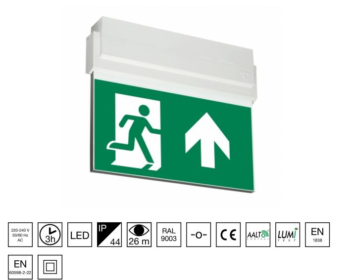
Self-contained LED Emergency Exit Light with 3 h Battery and Wireless Central Monitoring, with 2-sided pictogram, arrow up, 26 m viewing distance (Invidually packed TWT8053WA)
