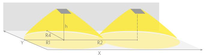
R1 distance from wall (X axis) R2 installation distance between lights (X axis) R4 distance from wall (Y axis) Y4352WM
