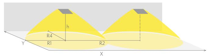
R1 distance from wall (X axis) R2 installation distance between lights (X axis) R4 distance from wall (Y axis) TWTA152WA
