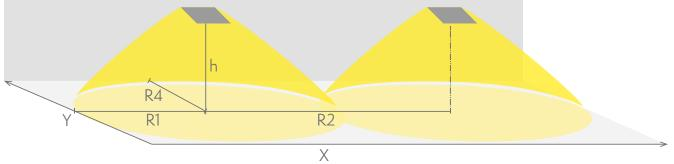
R1 distance from wall (X axis) R2 installation distance between lights (X axis) R4 distance from wall (Y axis) TWT9953WM
