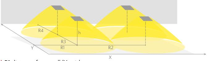
R1 distance from wall (X axis) R2 installation distance between lights (X axis) R3 installation distance between lights (Y axis) R4 distance from wall (Y axis) TWT3651WK
