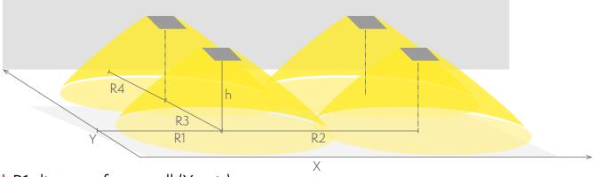
R1 distance from wall (X axis) R2 installation distance between lights (X axis) R3 installation distance between lights (Y axis) R4 distance from wall (Y axis) TWT3271W
