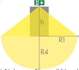
R1 distance from wall (X axis) R4 distance from wall (Y axis)
