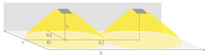
R1 distance from wall (X axis) R2 installation distance between lights (X axis) R4 distance from wall (Y axis) TWT2921
