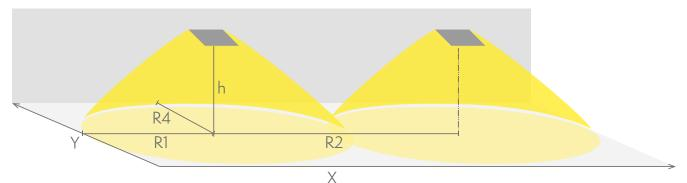
R1 distance from wall (X axis) R2 installation distance between lights (X axis) R4 distance from wall (Y axis) TWSC292WAC
