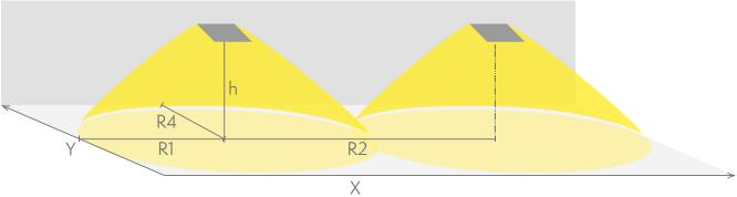
R1 distance from wall (X axis) R2 installation distance between lights (X axis) R4 distance from wall (Y axis)
