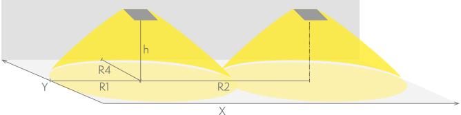
R1 distance from wall (X axis) R2 installation distance between lights (X axis) R4 distance from wall (Y axis) TWS4292WM
