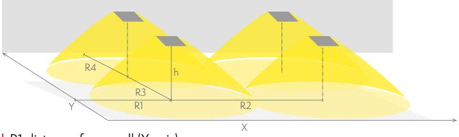
R1 distance from wall (X axis) R2 installation distance between lights (X axis) R3 installation distance between lights (Y axis) R4 distance from wall (Y axis) TWS3292WA
